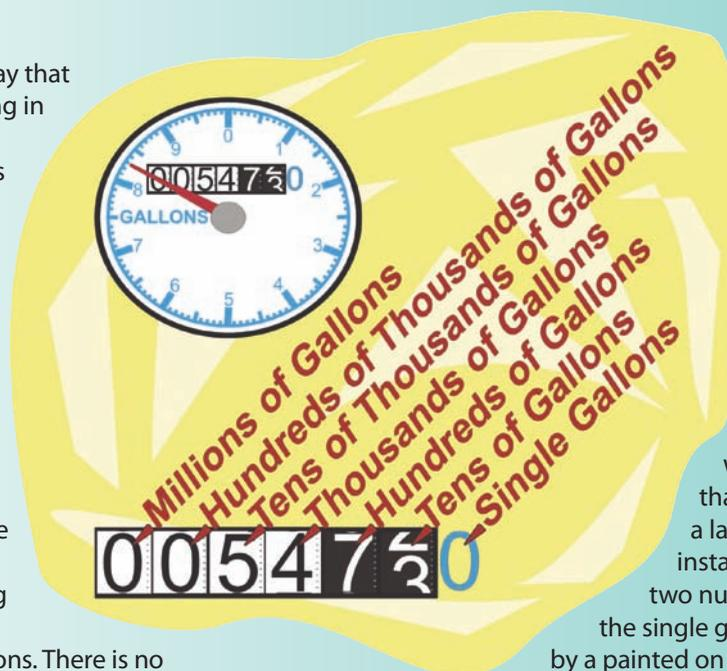
district had their software set up to enter meter readings down to the detail of the tens of gallons. Before the newly built school all of their customers had common residential meters that had the one painted on zero like the meter shown in the example so they would have entered that reading as 5472. As is often the case
