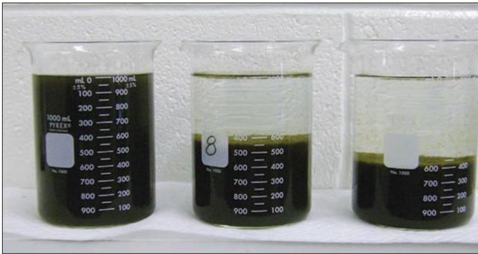
From L. to R.: Settling test results at 0 minutes, 15 minutes, and 30 minutes.
