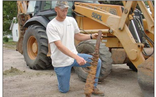
The city of Greenleaf experiences many breaks and leaks in its old steel water distribution system as evident from the clamps on this section of 3-inch pipeline held by City Employee Jerry Baker.
