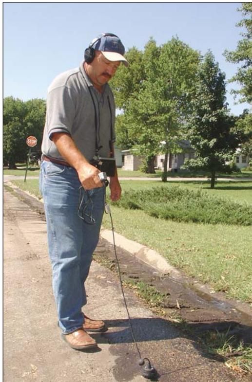
*Methods for detecting leaks in water distribution systems may involve using sonic leak detection equipment, which identifies the sound of water escaping a pipe. Pictured above, KRWA Tech Greg Duryea uses an ultrasonic listening device to detect noise on a pipeline*
