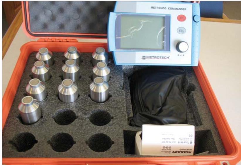
*This set of "data loggers" is but one of many devices KRWA uses to help locate water loss. The small cone shaped units are placed on valves, meter setters or any other part of the distribution system to detect system noise. Typically the units are programmed to turn on at 2 a.m. and then shut off at 3 a.m. The information from each unit is then downloaded into the Commander for analysis. Suspected leakage can then be investigated.*
