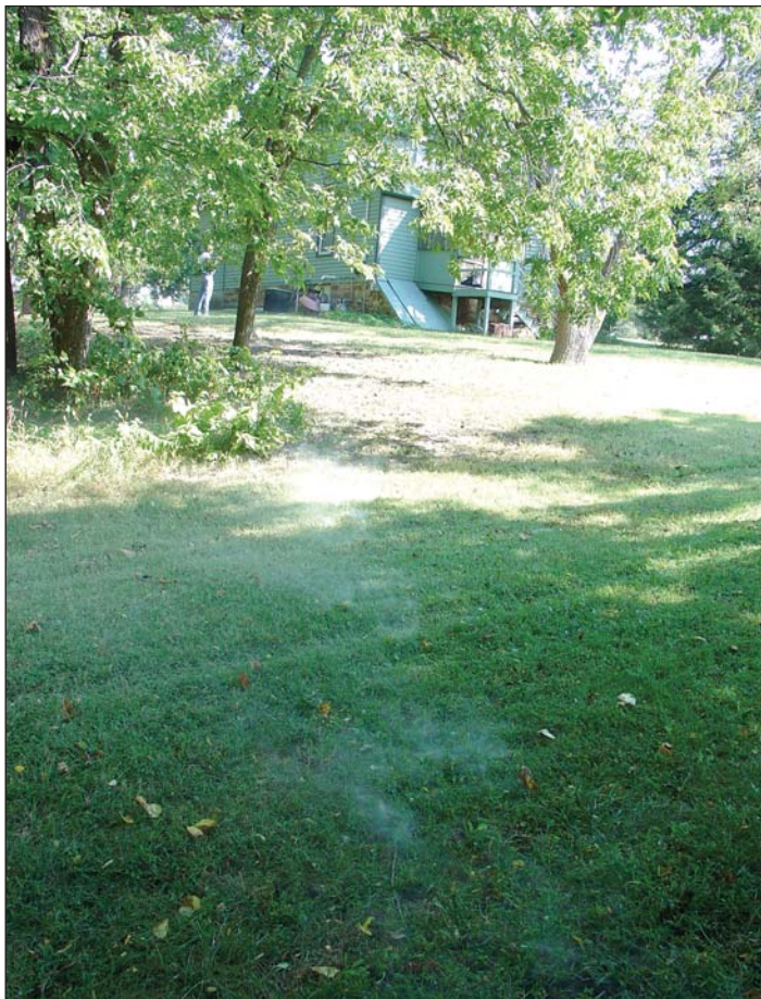
Smoke can be seen rising from the grass in this house yard. There is a break in the service line from the home to main. Breaks in service lines have been the most common problem found during smoke testing by KRWA.
