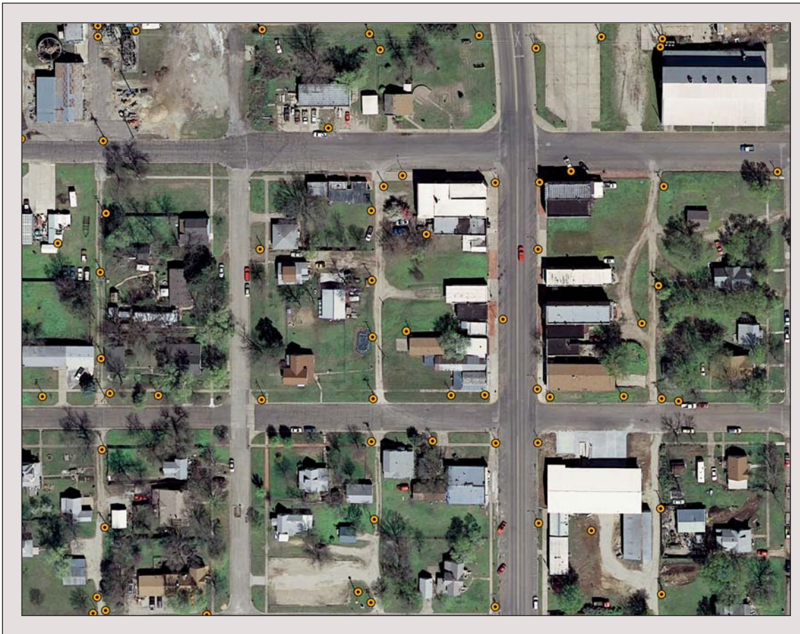
This map page shows power pole locations in Enterprise, Kan. The background is a 2007 high resolution aerial photograph of the city and surrounding area. This mapping system allows city personnel to quickly and accurately identify what poles are on which streets throughout the city.
