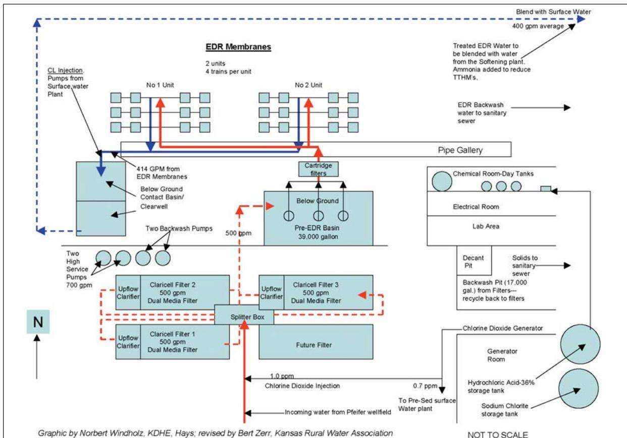
example, at the Russell plant, routine operation is to allow normal flow through the membranes for about 20 minutes followed by a one minute electrical ion exchange during the cleaning process. This process continues with part of the waste stream being returned and rerouted through the membranes.
