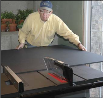
Above: A 4 x 4 ft. panel is cut to 32-in. wide with a table saw.
