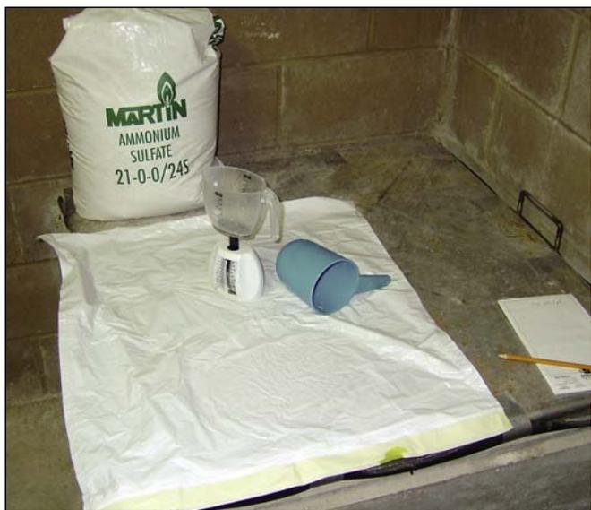
*The system's ammonium sulfate weighing process consists of cups, a surface to catch any spillage, a kitchen portion scale, pencil and paper.*
