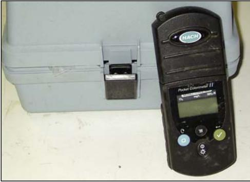
**Above:** Free ammonia levels in the water entering the pumping station are measured with the free ammonia and monochloramine tester.
