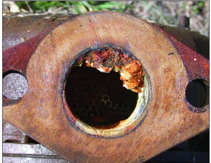
*This is what can happen if proper maintenance is not performed regularly on a system's meters. When tested this meter was over registering which led to the water system showing a water loss.*
