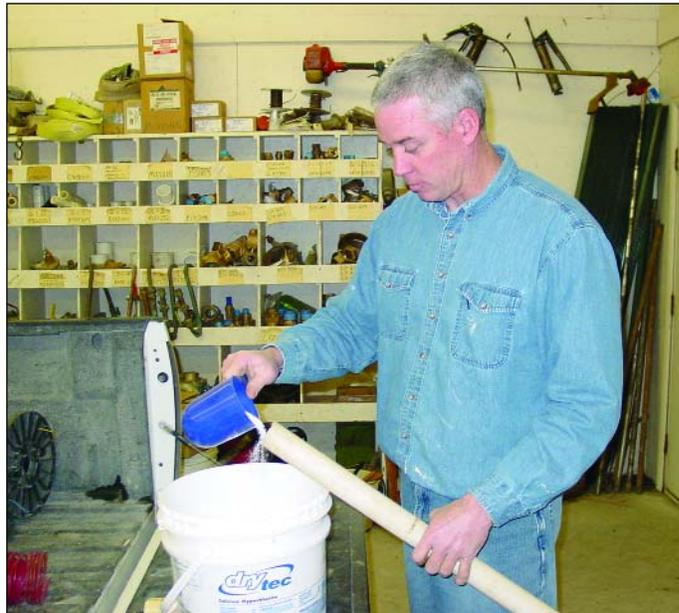
Nemaha RWD 3 Operator Paul Strathman fills his “portable chlorine container” from the bulk bucket that the system purchases to sanitize newly installed pipes. The short length of pipe is easily capped and fits nicely in a work vehicle.
