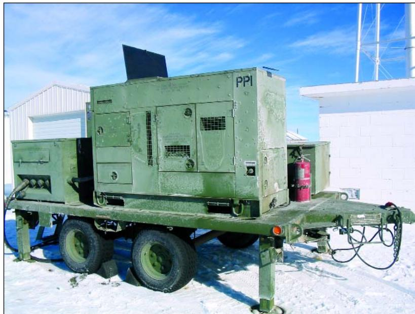
*This Kansas Army National Guard generator is hard at work in Park, Kansas. It is one of nearly 100 generators brought in to assist utilities in keeping services up and running during the area's recent severe ice and snow storm. Generators were taken back to the Hays armory for repairs when needed.*
