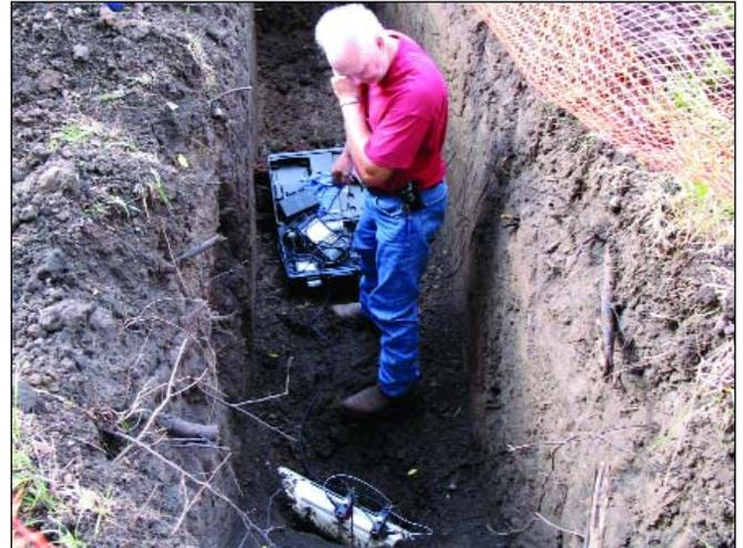
*KRWA Technical Assistant and Training Director Gary Armentrout uses an ultrasonic meter that not only gives the rate of water flow in the pipe but also shows the direction of water flow.*
