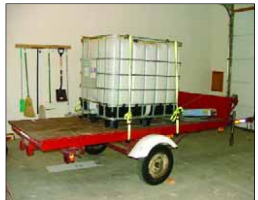
Trailer mounted storage tank used in the process for super chlorinating system wells.
