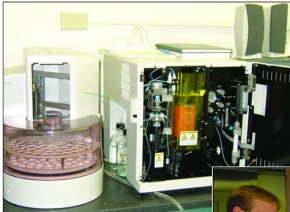
**Right:** KDHE laboratory instrument for persulfate-ultraviolet oxidation for TOC analyses.
