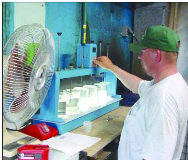
Carbondale operator Kevin Richardson performs jar testing to adjust coagulant feedrates to attain the best possible finished water.
