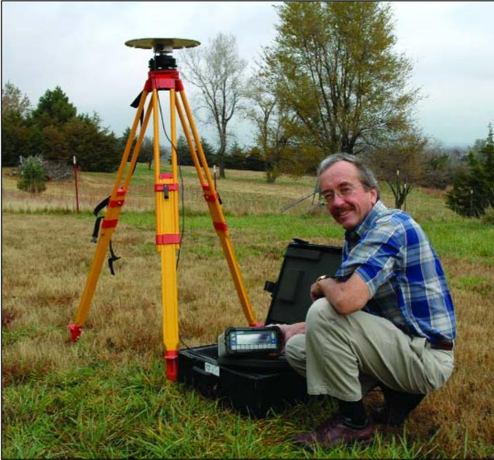
*Steve Thompson sets up a survey and engineering grade GPS receiver, which allows centimeter level measurements and locations. This same GPS receiver with radio equipment, not pictured, is also capable of centimeter level navigation used in construction staking.*
