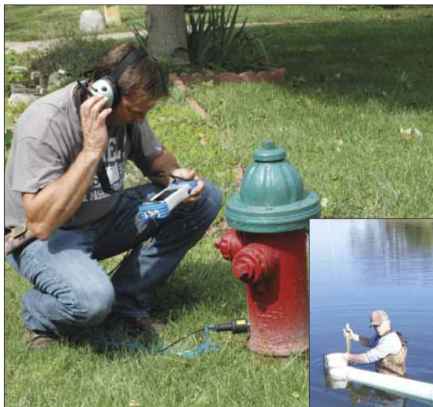
Greg Metz, Technical Assistant listens to fire hydrant for water loss at Manhattan, Kans.
