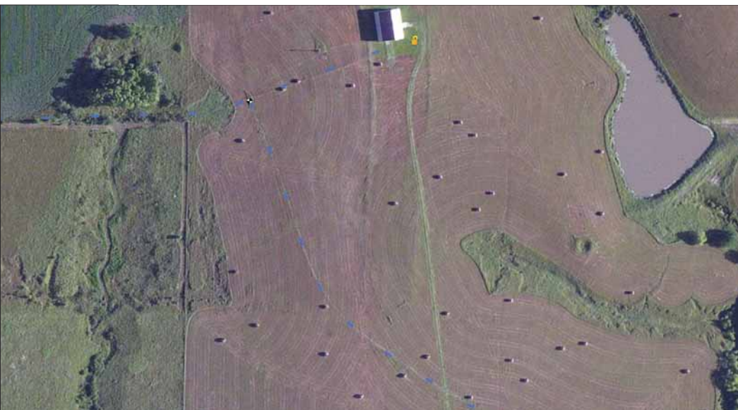
The blue dashes indicate the location of another "cross country" water line in Morris County. The trench line is very apparent in this aerial 2021 image. The pipeline was installed a few decades ago through native tallgrass prairie.
