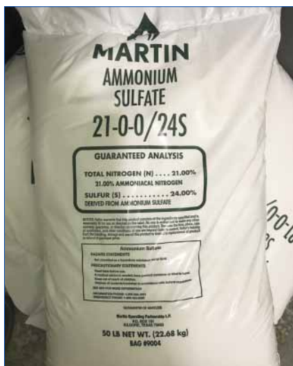
Most surface water treatment plants add ammonia to form chloramines and limit DBP formation.
