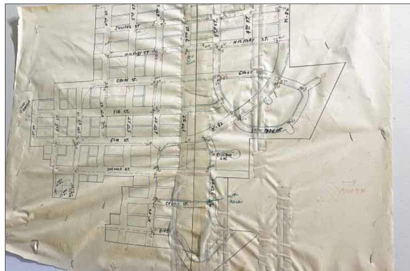
This is the only map of the water system that the operators in the city of Wakefield have ever known. It is completely hand drawn on a vinyl sheet; most valve locations are inaccurate.
