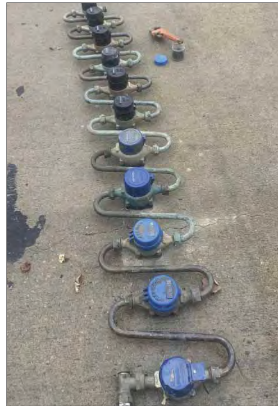
Testing a sampling of customer meters is a part of thorough water loss survey. This photo shows meters from a water district connected in series to save time on testing.
