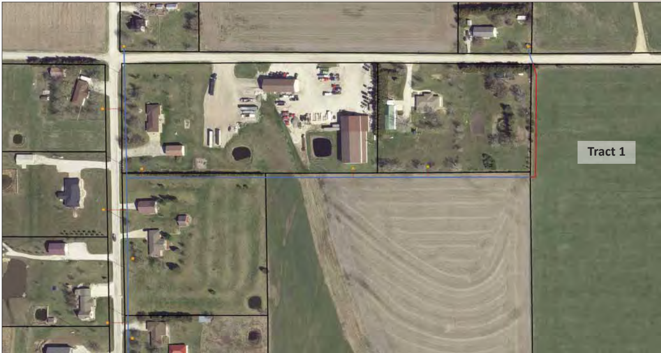
The blue line represents a water line that provides service to nine homes (meter locations indicated by yellow dots). The blue line is all located in recorded easements on private land. The red line represents that portion of the water line that transports water to the single customer (blue line) and is located on a separate tract of land with no easement (Tract 1).
