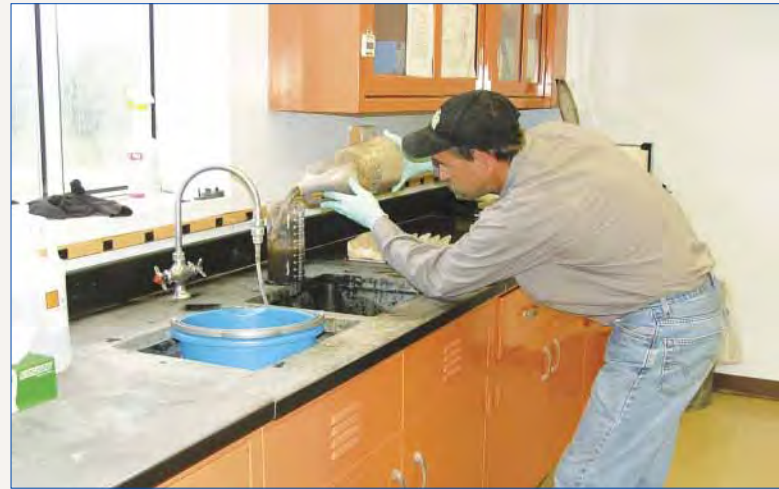
Utilities that operate mechanical wastewater plants conduct a range of tests every day. This operator is conducting a settleability test. The test is an analysis of the settling characteristics of the activated sludge, mixed liquor suspended solids (MLSS).
