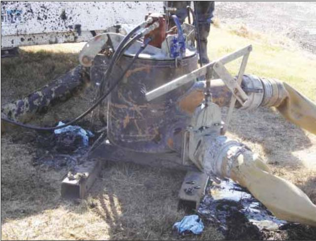
**This grinder pump was used to grind rubber and plastic products in the sludge so that such materials do litter the land application site.**
