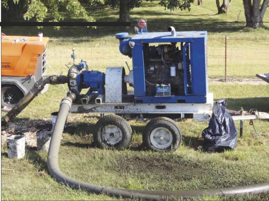
An intermediate booster pump was used to pump sludge to the land application site. It was located downstream of the pump powered by a tractor power-takeoff located at the corner of the cell being desludged.
