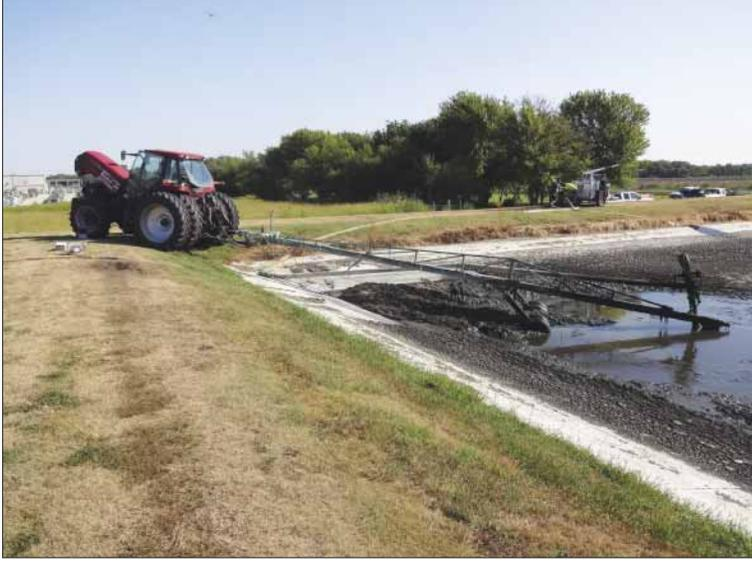
This photo shows the pump located at the corner of a cell powered by a tractor. Sludge is directed to a grinder pump and then the intermediate booster pump before reaching the application site.
