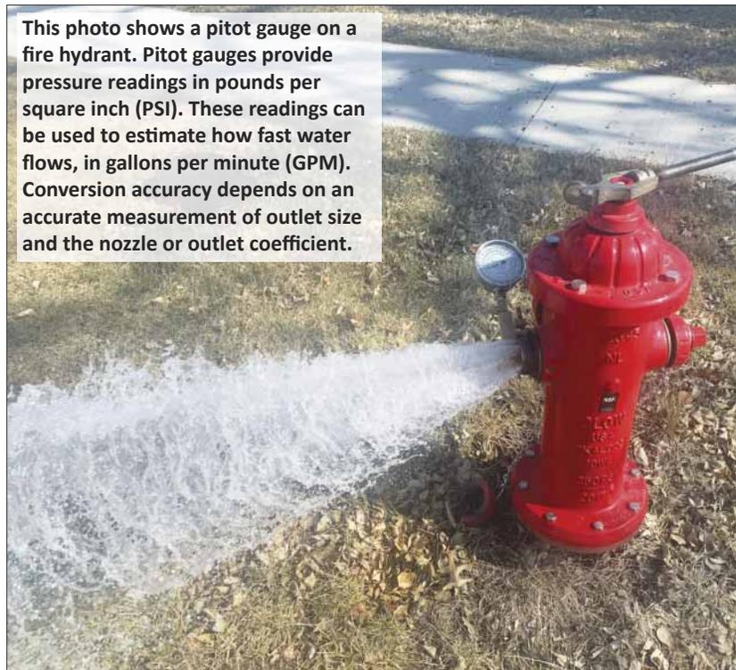
This photo shows a pitot gauge on a fire hydrant. Pitot gauges provide pressure readings in pounds per square inch (PSI). These readings can be used to estimate how fast water flows, in gallons per minute (GPM). Conversion accuracy depends on an accurate measurement of outlet size and the nozzle or outlet coefficient.
