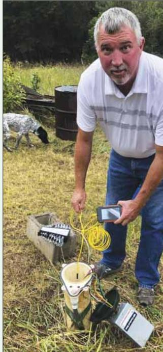
**The photo shows KRWA Tech Assistant Lonnie Boller testing drawdown in a privately-owned well in mid-September 2022. KRWA's newest gauges prove a method to also collect video of the well.**
