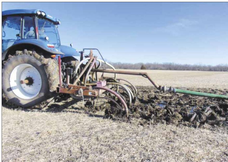
**These photos show sludge being pumped from a lagoon to a tractor pulling an injector in a soybean field.**
