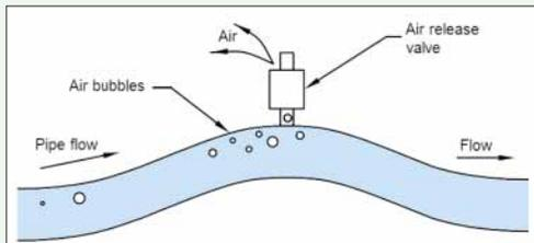
This graphic illustrates the proper location of an air release valve.
