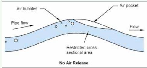
Air in a waterline generally forms on the downhill side of the highest point. This is because of the flow of water in the pipe. Air enters pipelines on startup following installation or shutdowns due to repairs.
