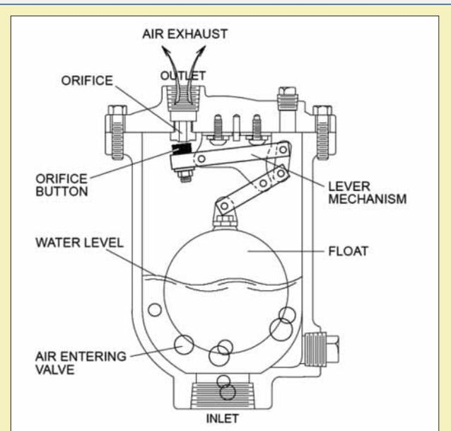
The air release valve is designed to automatically remove air pockets at the high points in a piping system. The valve, as shipped, is a normally open valve and will slowly vent air through the top orifice. The float will rise as fluid enters the valve, closing the orifice. As air accumulates in the piping system and enters the valve, the float drops, allowing the venting orifice to open.
