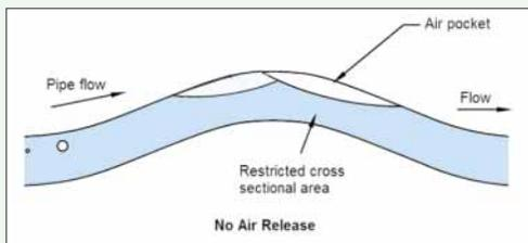
Air in a waterline can result in flow restriction to the point in severe cases of entirely blocking the flow of water. When the air becomes dislodged, water hammer can result as the air may separate and surge forward, causing tremendous pressure differential in the pipeline, resulting in breakage of pipeline or fittings.
