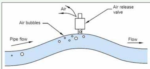
Air release valves open against internal pressure because the internal lever mechanism multiplies the flow force to be greater than the internal pressure. This results in the orifice opening when air pockets collect in the valve.
