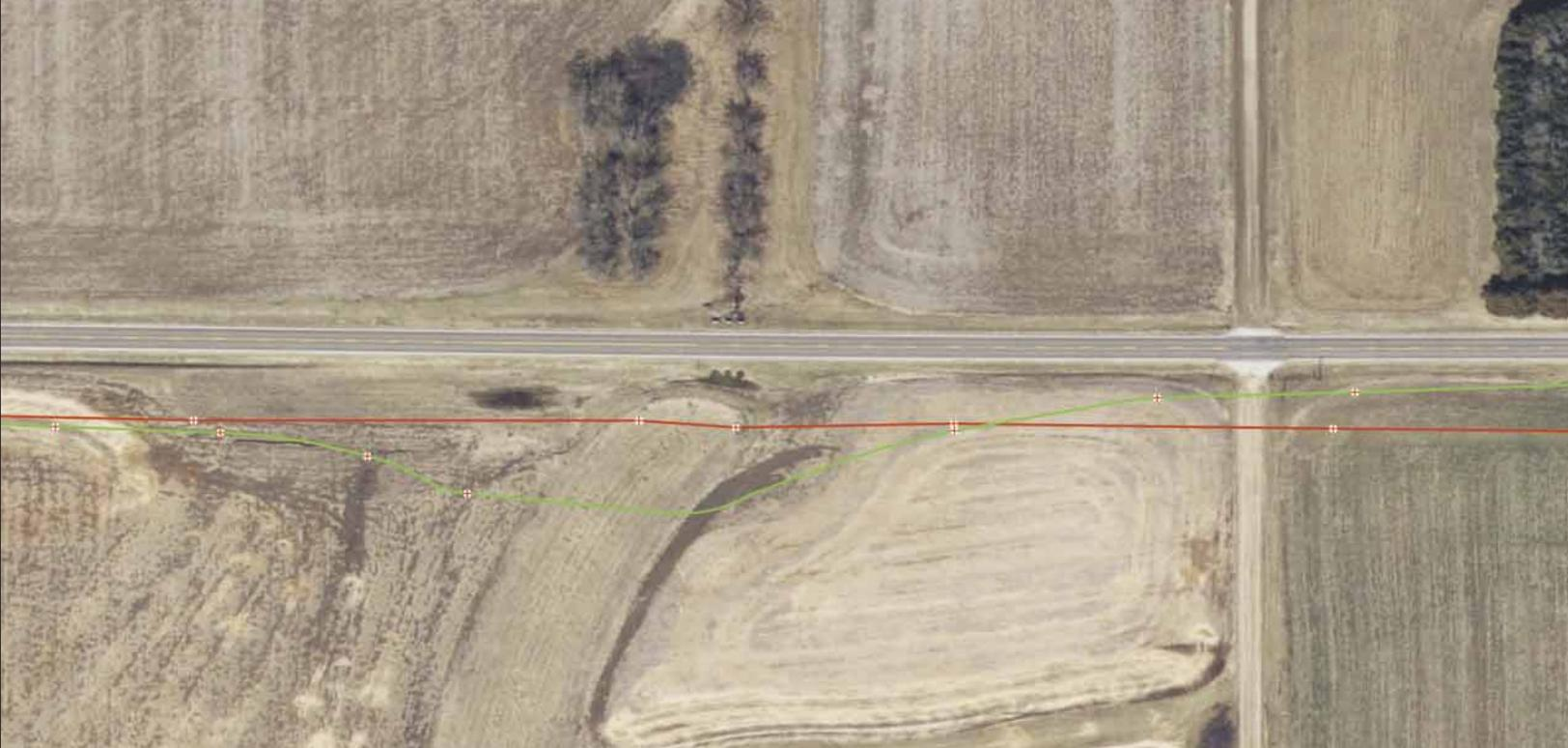
This graphic shows the installation of a newer 6-inch waterline (red) in Washington RWD 2 near Linn, Kansas. The green line is the original 4-inch line installed in 1985. It was necessary to locate the 6-inch because of roadwork to replace a bridge.
