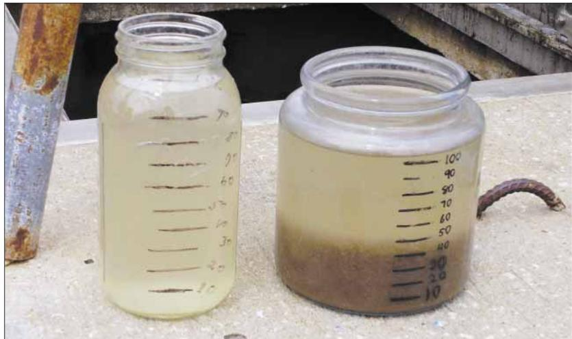
These are examples of old glass containers that have been adapted for running settleability tests and monitoring sludge depths at 5-minute intervals. Note both are very cloudy. The one on the left appears to be a Mason jar.
