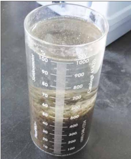
This settleability test just ended at 30-minutes. Note the sludge depth of 50 percent. The supernatant is relatively clear with a few straggler floc. The color of the sludge is also very good with a chocolate-brown color.
