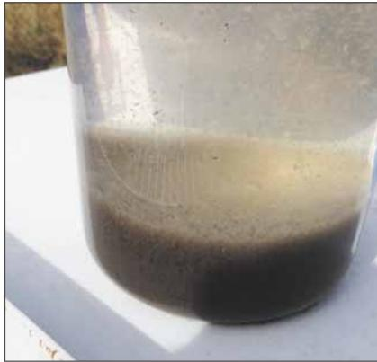
**The sludge layer is a good brown color and has consistency. It's not extremely compacted like an old sludge, but not fluffy like a younger sludge. While a few stragglers are left behind in the supernatant; the operator did not use a clean beaker.**
