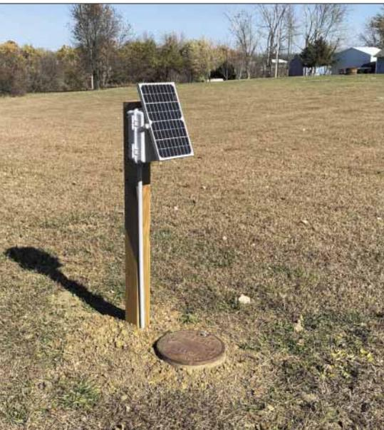
**RPM20 Deployment in the field. This model has a solar module, a battery and battery charge controller. It can be deployed just about anywhere.**
