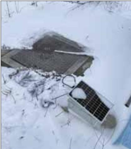
Emergency deployment of the RPM20 at Leavenworth RWD 9 during the February cold spell provided them tank pressure data after the line to their SCADA froze.
