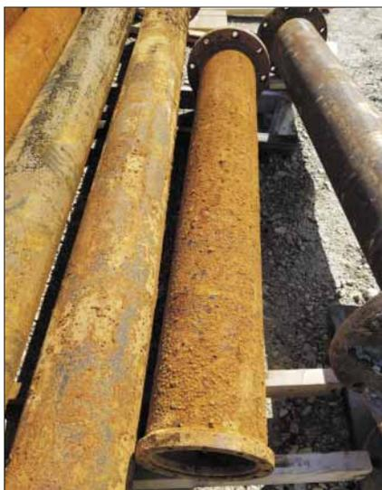
This is a photo of the column pipe showing corrosion inside and out along with biomass buildup.
