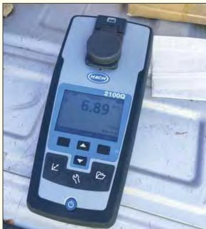
KRWA's 2100Q portable turbidimeter, being used to test the effectiveness of each jar.
