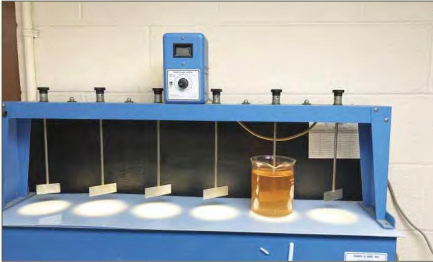
This photo shows a jar tester being used to check permanganate dosage for the control of manganese.
