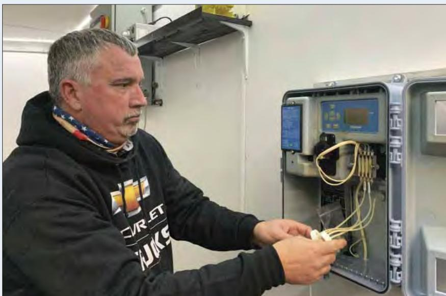
KRWA Surface Tech Lonnie Boller checks the tubing on CL17 Analyzer after installation in the new training trailer being assembled by KRWA.
