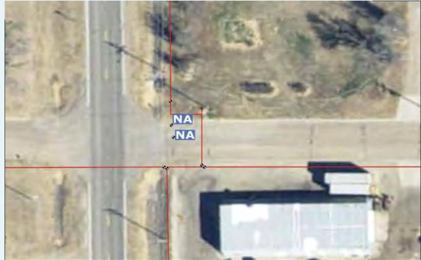
**This image is of 4th & A Street. The two valves in the street marked "NA" are not active. These are examples of valves not removed during a system improvement project years ago.**
