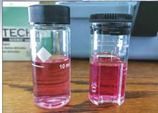
The differences in the low range glass vial (left) and the high range plastic vial are shown here. Low range analyses require a 10-mL sample while high range requires a 5-mL sample.
