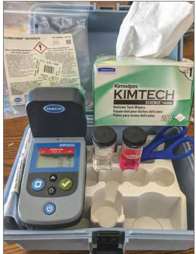
The author's colorimeter kit is shown here. A small pair of scissors will be handy to open reagent packets when hands are wet.
