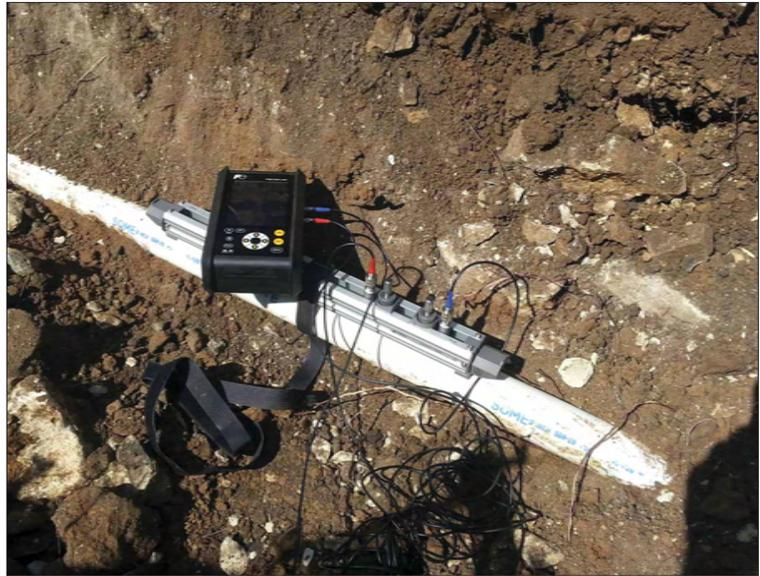
KRWA has two of the Fuji Portaflow ultrasonic flow meters. This photo shows one of them in use on a small water line in a rural water district in an attempt to isolate a leak. This non-invasive meter measures the velocity of water with ultrasound to calculate volume flow.
