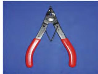
Joint Restraint Pliers
