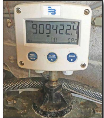
Chapman uses digital displays for the meters on their water wells. The large digital displays help provide accurate records of water diversions.
