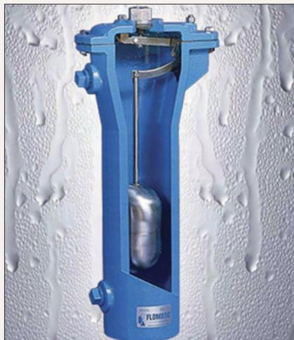
The typical difference between a water or wastewater air relief valve is that, as shown here, the wastewater devices are normally taller to prevent the solids and wastewater from being released.
