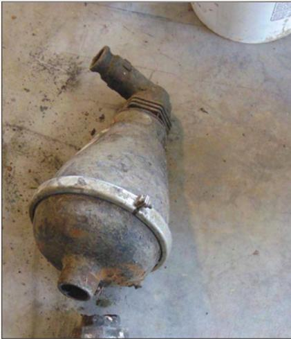
**Galvanized fittings were used for the original installation of this air relief valve. Severe corrosion resulted in a leak. A plastic fitting will replace the corroded fitting.**
