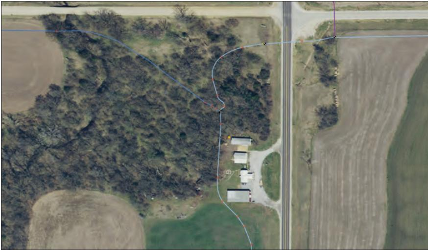
**The graphic shows the district's water lines KRWA collected in April 2020. The pipeline is installed behind an old service station. A leak on the original 2 ½-inch line caused the district to replace the line in this area due to the terrain and knowing that more leaks would surely occur. Washington RWD 1 has been plagued with many leaks on solvent weld pipe since it was installed in the mid-1970s**
