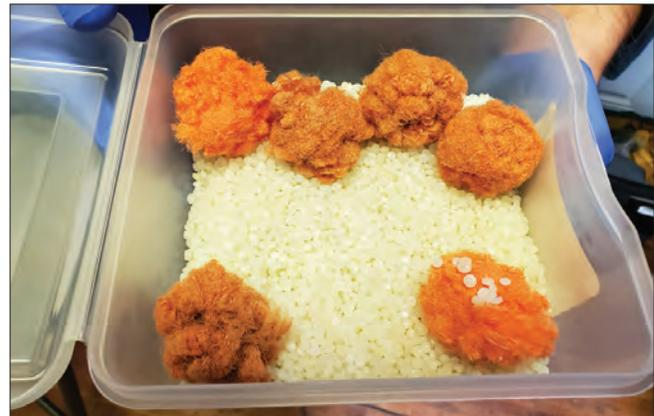
Compressible and buoyant media in adsorption clarifier.
