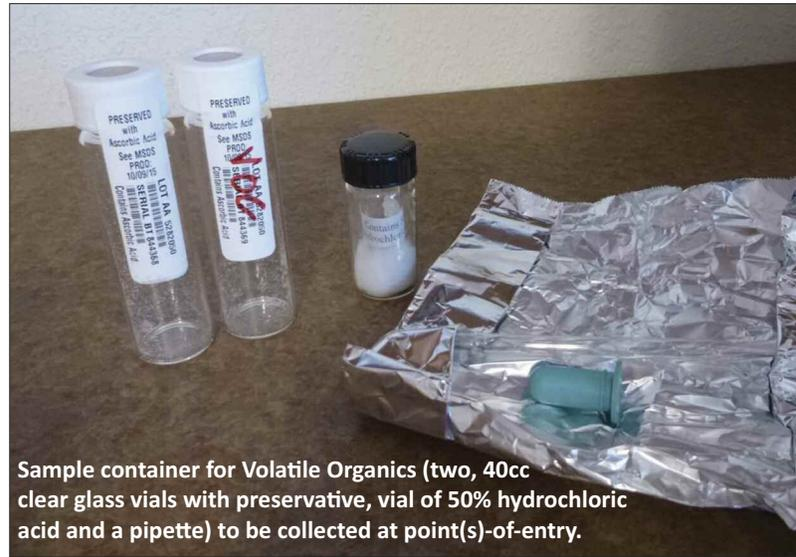
Sample container for Volatile Organics (two, 40cc clear glass vials with preservative, vial of 50% hydrochloric acid and a pipette) to be collected at point(s)-of-entry.
