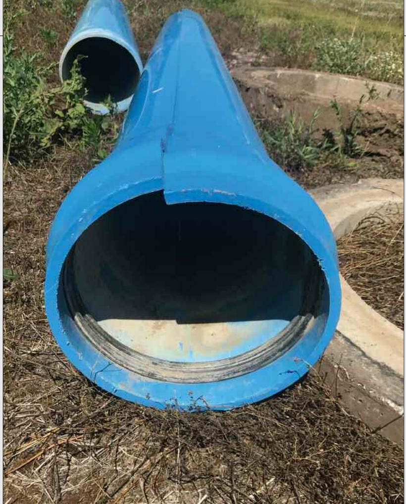
Section of 10-inch pipeline with longitudinal split. The cause of these splits has not been determined but was the cause for the city to install 5,500 feet of new CL 250 PVC pipe.
