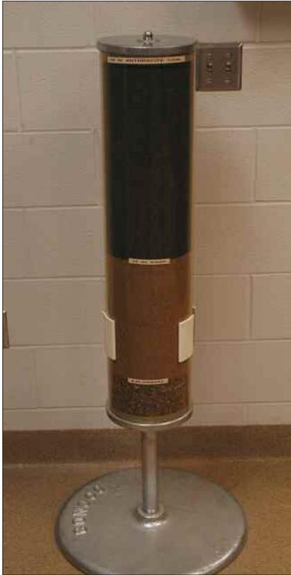
This model shows a cross section of the filter media with four inches of gravel at the bottom, twelve inches of sand above the gravel, and eighteen inches of anthracite coal at the top.
