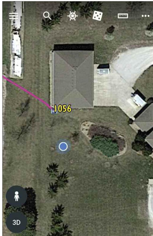
**This example of a location using a cell phone. The blue dot is the location of the phone. The actual meter location is at the corner of the building. The free app helps an operator determine the locations of infrastructure.**
