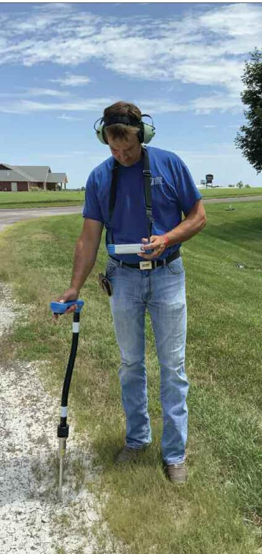
A focus of KRWA's work is to help water systems reduce unaccounted for water. KRWA Tech Greg Metz is shown using the latest sonic leak detector in KRWA's equipment inventory – a new SebaKMT (HL 7000) ultrasonic unit.
