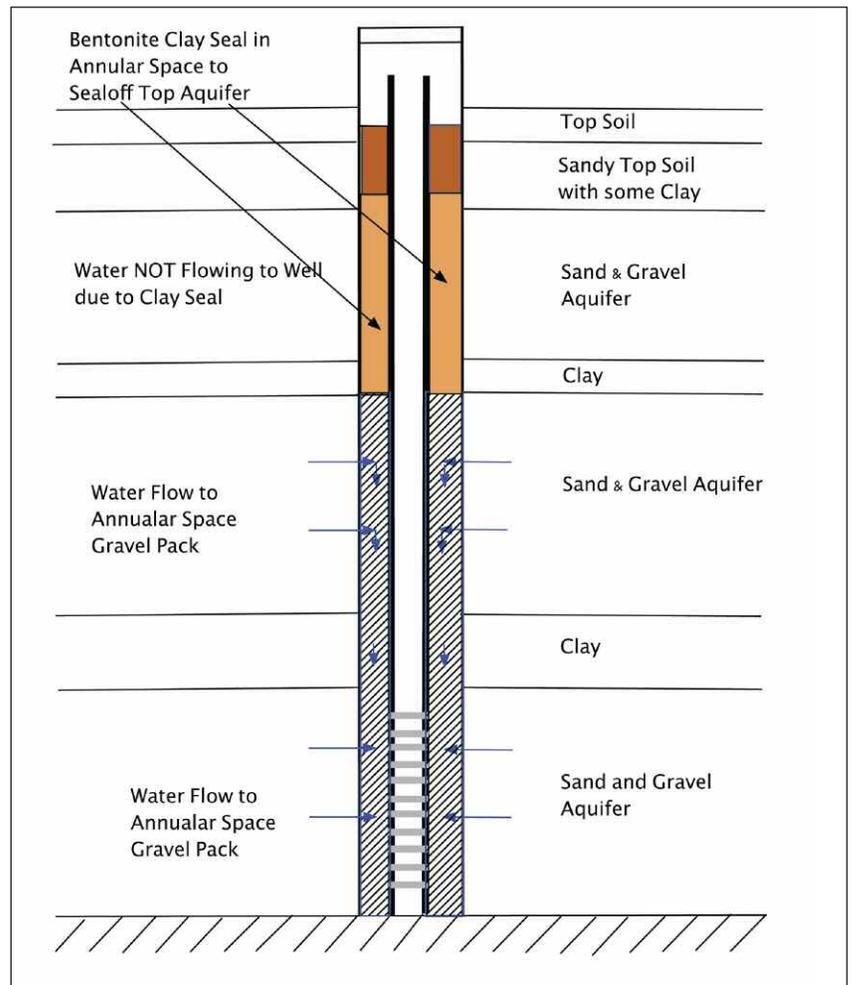
This drawing shows the same well design concept as Schematic A except the gravel pack is not continuous from near the top to the bottom of the well casing.
