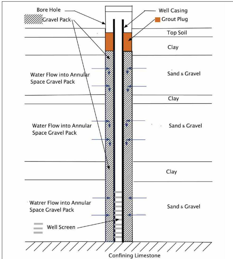
This schematic shows a well that receives water from three different aquifers.
