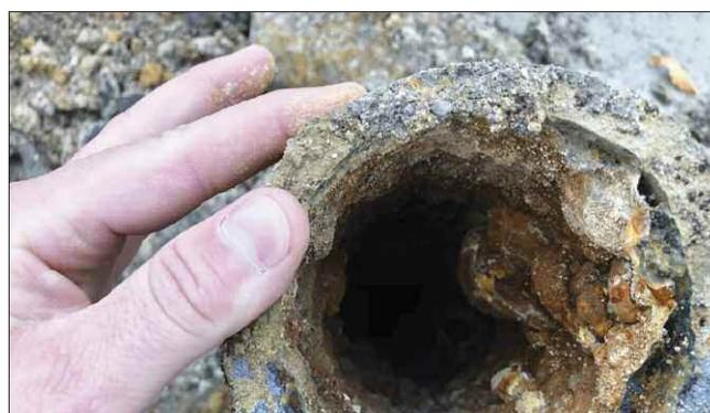
This section of 4-inch pipeline shows extensive buildup of mineral deposits in the existing water distribution system in Washington, Kansas. The city is embarking on a total replacement of the system.
