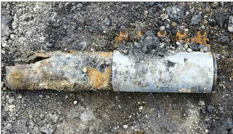
This cutout of a 4-inch cast iron pipeline shows a new break just adjacent to a clamp that repaired a prior break.
