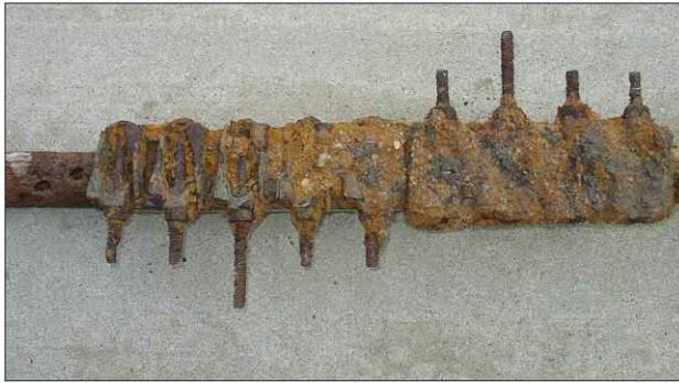
Pipe from a water system in Kansas. Many clamps....
