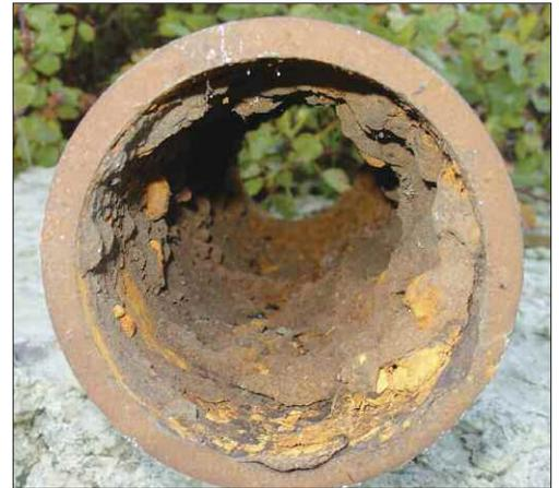
This section of 4-inch cast iron pipe shows excessive mineral deposits found in many old water lines.
